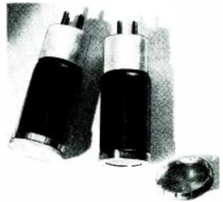
Tracerlab tubes with removable beta shields.
