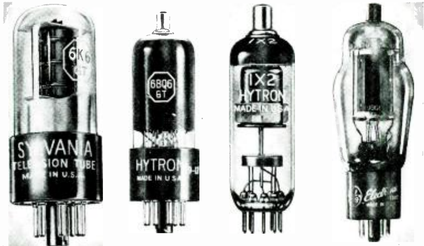
Photos 1, 2, 3, and 4—Sylvania television tube, Hytron 6BQ6-GT and 1X2, and G-E 19BG6-G.
