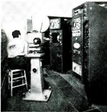
Fig. 1—Photographing the monitor. Edge of a monitor tube may be seen in the rear rack.
